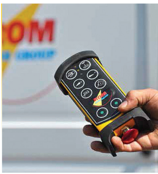
Electrical radio remote control Professional-Remote, 7-channels
