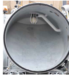
Slanted bottom system; fast and quick unloading and cleaning of tank
