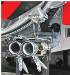
Integrated (forklift) tubes; ideal for hose storage
