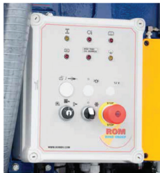
Control box at engine/pump combination (ROM SmartCombi PRO)
