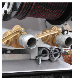
Discharge valve + Suction valve
