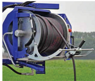
Extendable hose guiding system with bearing
