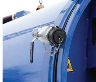
Drain pipe for draining water from the waste water tank
