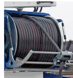
Flexible and kink resistant sewer cleaning hose with wear- resisting, smooth exterior; slides through bends easily
