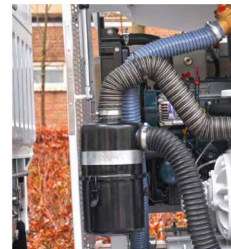
Combined oil separator / silencer (Vacuum pump version)
