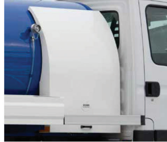
Lockable design engine / pump compartment cover, (standard carmine red RAL 3002)
