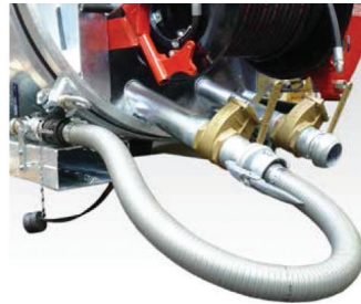
Linking system for the waste water tank on to the fresh water system
