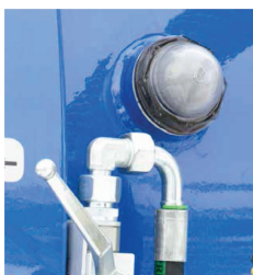
Level indication via sight glasses in tank body (sludge)
