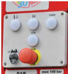
User friendly water-resistant control panel (ROM SmartCombi)
