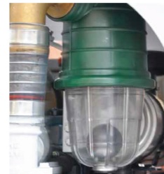
Moisture guard; for optimal protection of the vacuum pump (Vacuum pump version)
