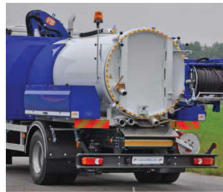
Larger tank capacities fresh and sludge water; 3000 litres in total
