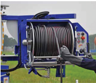
270° rotating hydraulically driven HP reel, mounted on swiveling frame
