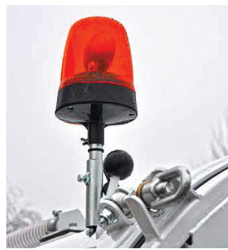
Rotating beacon on pole
