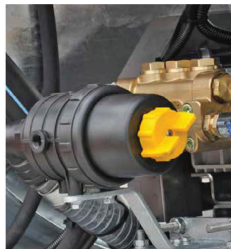
Automatically closing water filter with rinsable element
